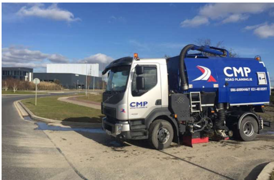
Figure 5-1: Typical Road Sweeper (Source: CMP Road Planning)
