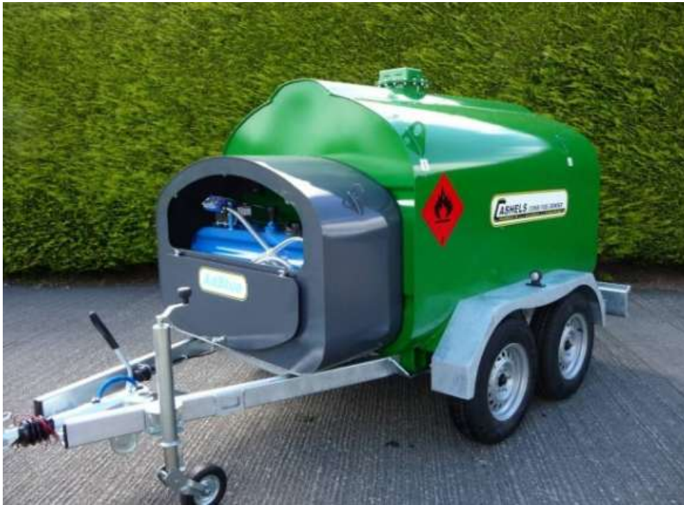
Figure 4-3: Typical mobile fuel bowser (Source: Clarke Machinery Group)
